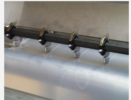
The films cut into strips are then cut to the desired length by a cross-cutting module. During the design phase, particular emphasis was placed on quick knife changes.
