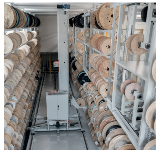
Robotic and MES controlled reel handling
