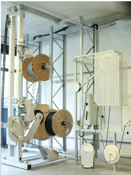
Cable rack with automated cable reel handling
