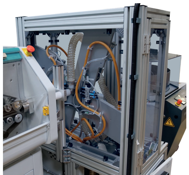
Cable cleaning unit with brushes
