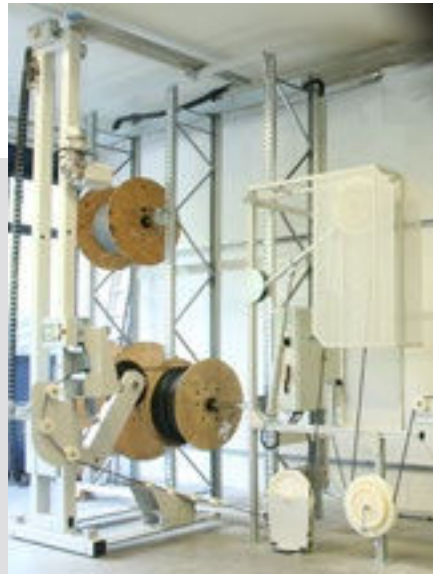
Cable rack with automated cable reel handling
