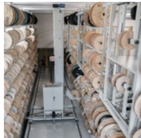
Robotic and MES controlled reel handling
