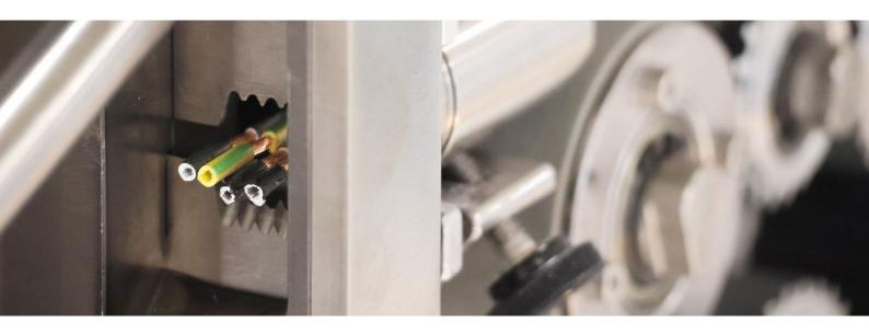
When processing multiconductor cables there is often the requirement to process also the inner conductors together with jacket stripping.
