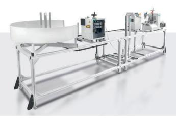
A wide range of 100% compatible Metzner unwinders, feeders, winders, stackers and printers are available for the Metzner ST-OB.
