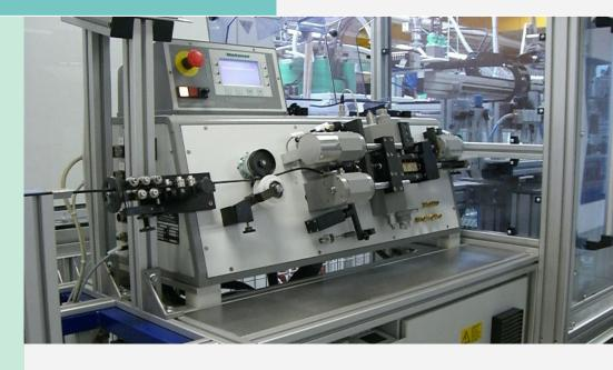
roughened to an exactly defined depth. In addition, a camera system must check and record the various work steps. Finally, the processed cables must be transferred to a workpiece carrier system fully automatically and with high precision.
