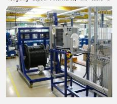
stripped at the desired place. The system requires 4.5 seconds for the entire cable processing, incl. depositing. All parameters, such as cable length, roughing depth or printing, are freely programmable and can be
