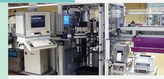
cable harnesses are either directly installed in the railway vehicles in the hall or are wound up and delivered to other assembly halls. For optimum production, integration in the existing IT network is necessary. This way, existing CAD data can be imported and, in combination with special Metzner software, all data for assembly generated – with optimised set-up times and order-specific.
