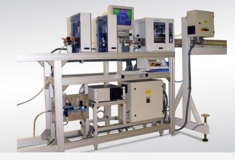
efficient way, all processing parameters can be called up at the push of a button via a PC program which is connected to the ITnetwork online. Based on this, the cables are then processed at any length and with cutouts at every desired position.
