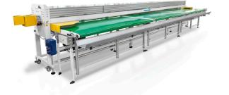
High-speed take-off by double ejector with front and rear take-off and integrated end sensing function.
