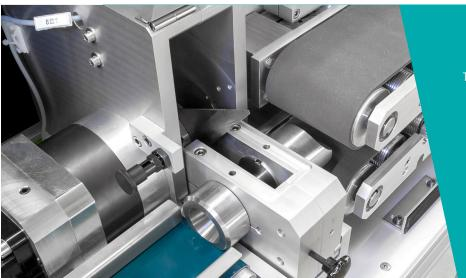
The cutting knife works in a fully enclosed working space. This not only gives working protection but also allows both wet or dry cuttting. With certain rubber compounds, it is essential that the knife is moistened and cooled to achieve a quality cut. Metzner Dynamat machines are equipped with this facility as standard.
