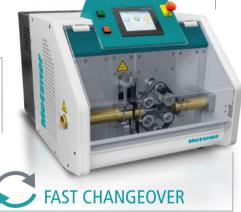
When frequent material changes are necessary, short changeover times are particularly important. Thanks to the Metzner »Quick Change System«, which assists in rapid guide changing, material changes are performed easily and without significant downtime.
