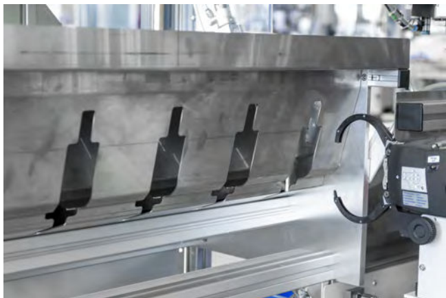
The line can bundle up to 54 cables on 17 freely selected positions.
