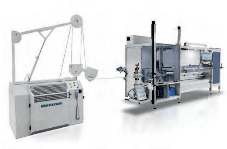
The cable processing line
