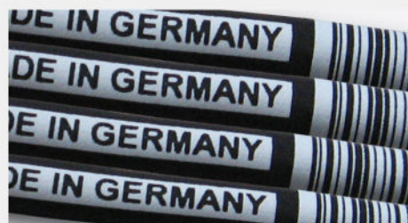
Fig. 2: Thermal transfer printing
