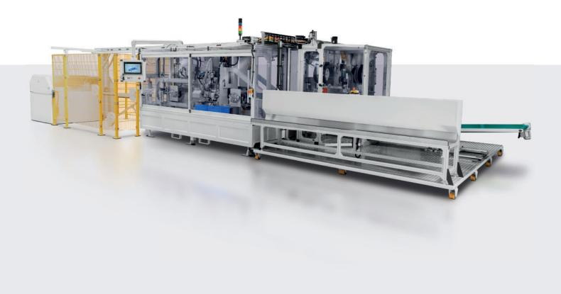
Due to their unique design, high-frequency coaxial cables call for very different processes compared to standard coaxial cables. Metzner developed the required process stations for those cables and integrated them into an automatic processing machine for cable preparation results shown below.
