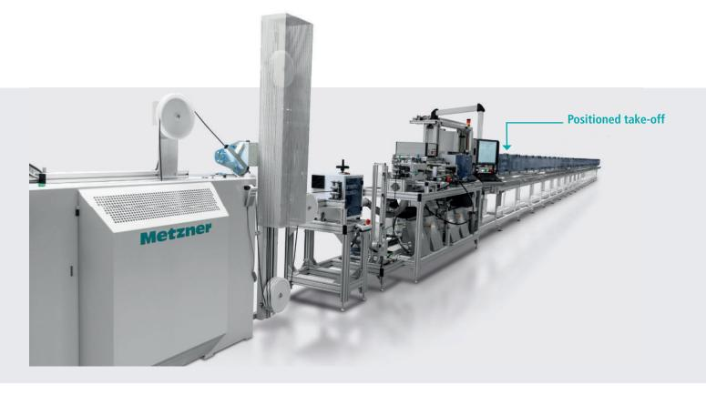
Automatic cable preparation for railway carriage harnesses; marking with modified ink-jet process that meets the durability requirements of the railway industry
