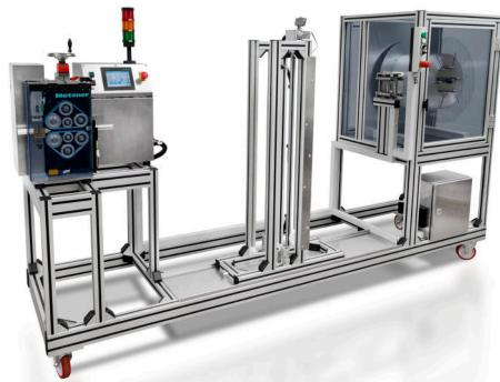
The Metzner KL-BV is also available in stainless steel, here in a production line with loop control and dereeler
