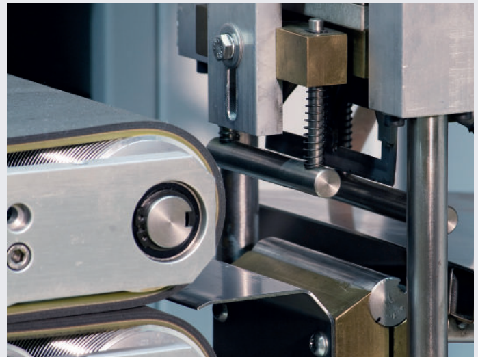
The MBS can be equipped with different tools. The picture shows the hot cut tool
